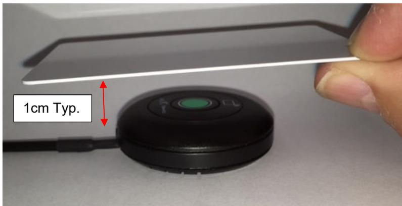
**Note:** DriveMate is NOT compatible with low frequency proximity card systems using 125kHz such as HID, PAC etc.
