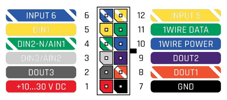
Figure 2 device 2x6 socket pinout
